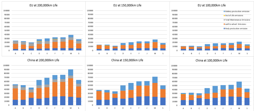
Figure 31 BEV LCA contribution in kgCO 2 eq of different stages for EU and China
