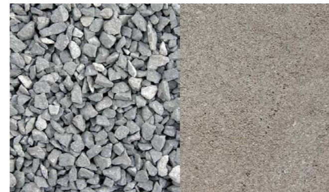
Screed made from recycled aggregates
