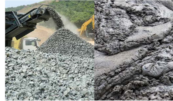
Low carbon cement with local recycled crushed aggregates
