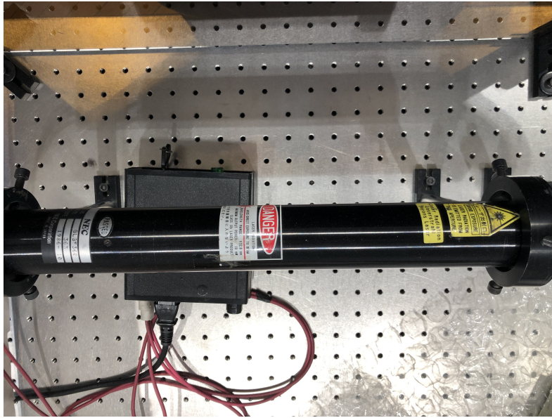
Figure 1.15: Photo of the He-Ne laser used in the laboratory.
