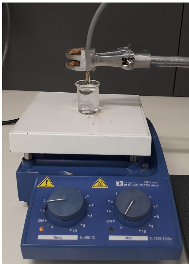
Figure 4.8: The experimental setup for evaluation the feasibility of dopamine concentration measurement by positioning the microelectrodes inside the solution and using magnetic stirrer to have a uniform solution during analysis. This setup can be improved by designing a system to hold the microelectrodes in an accurate position.
