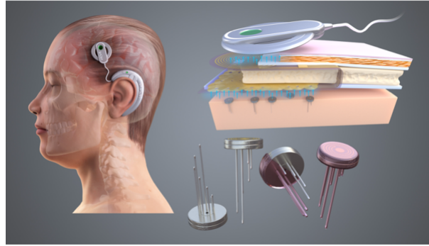
(a) ENGINI System: power supply, transceiver and probes.
