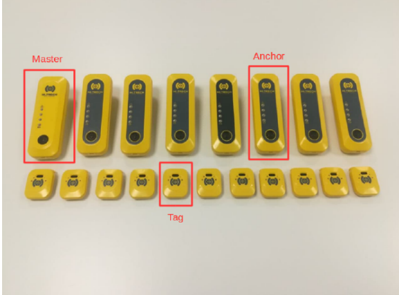
Figure 1: T4F system: the red boxes indicate tag, anchor and master anchor.
