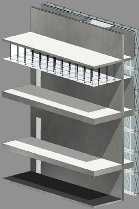
Figure 57: 3d section for the Facade system
