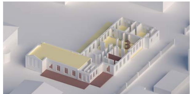
Figure 122: Ground Floor Demolition and Addition
