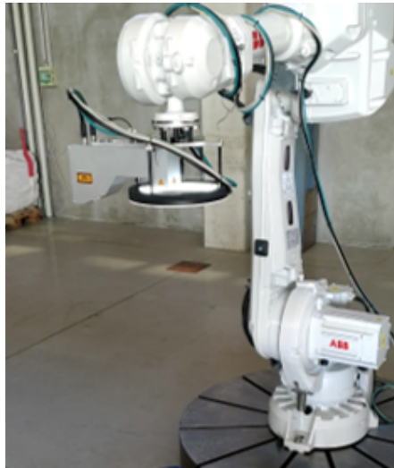
Figure 7.2: Robotic arm set-up for a future validation of the conceived approach in an industrial environment.
