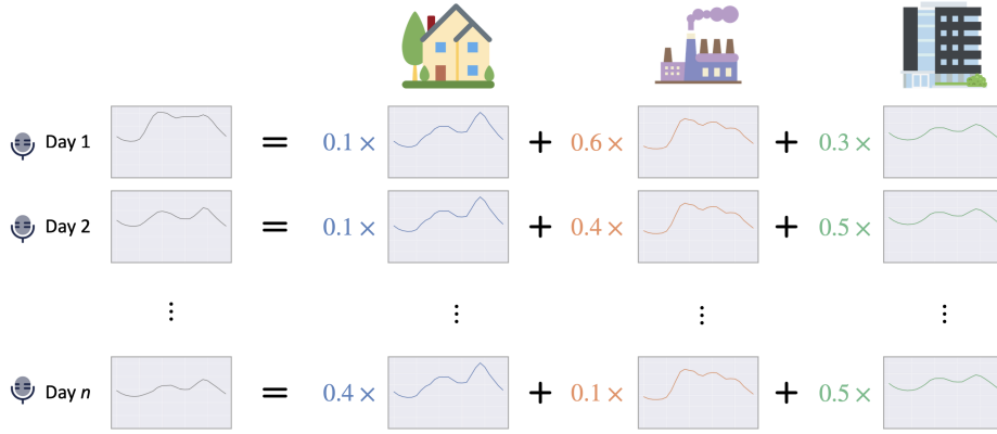
Figure 1.3: Illustration of the load disaggregation problem. In this example, each sector is associated to one source only.
