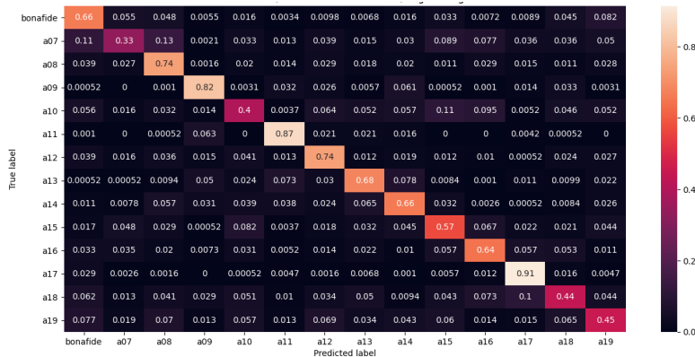
Figure 15: Confusion matrix of a multiclass classification (CSM) that involves the MKU features, performed using a series of one-versus-the-rest logistic regressions.
