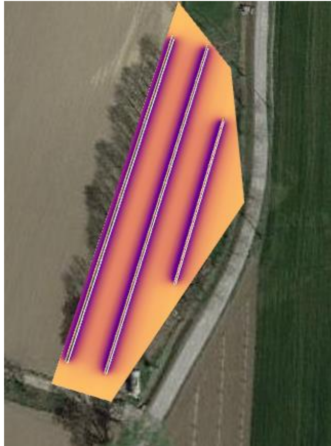
Figure 37: Rendering of the solar radiation incidence – Purple/dark equals lower than 50% - Yellow equals normal incidence.
