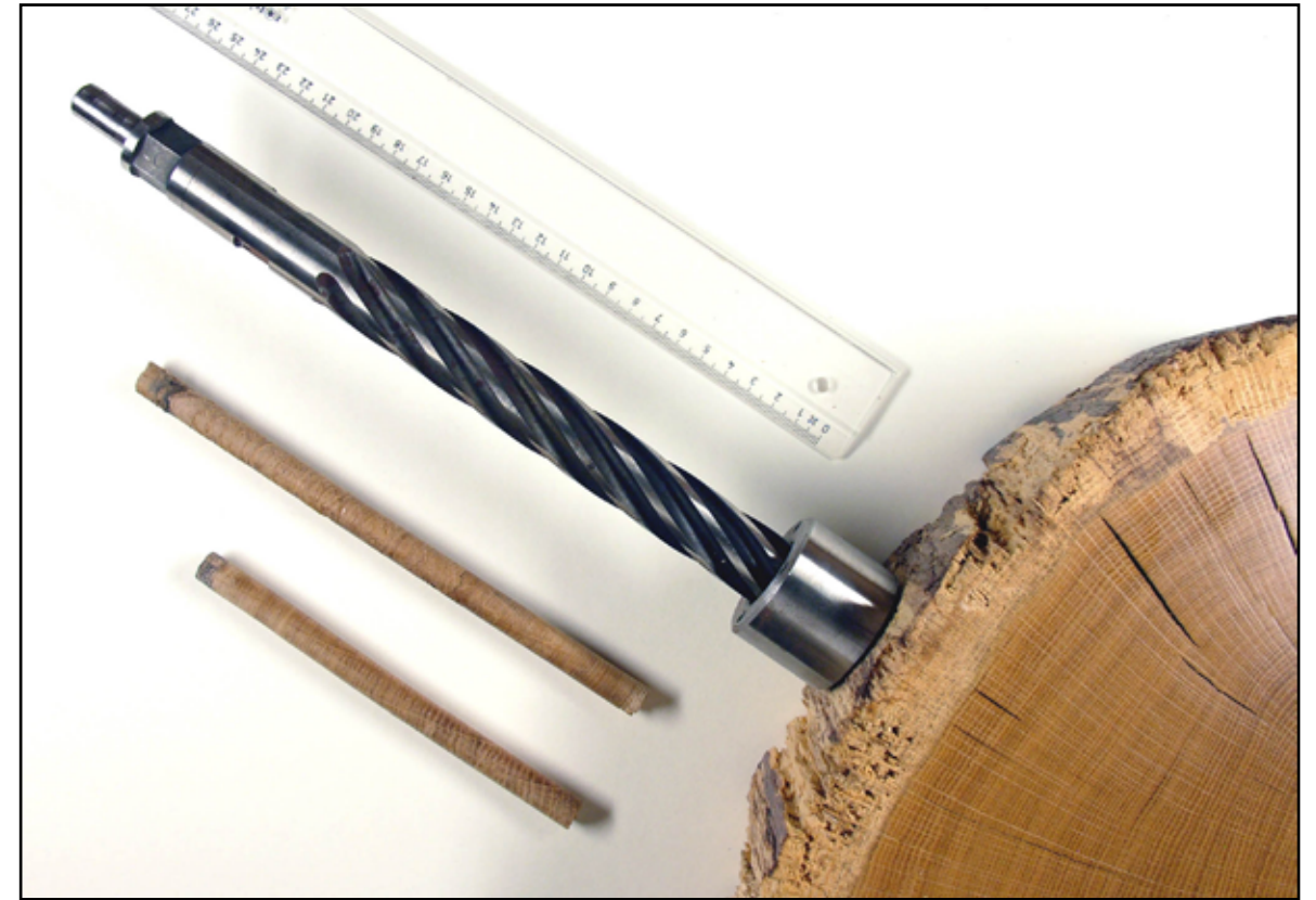
ILL 087 increment drill, used to extract dendrochronological samples
