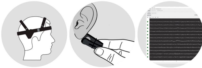
Fig. 98. Bitbrain EEG headset with example of the signal (Diadem | Wearable Dry-EEG Headset, n.d.)
