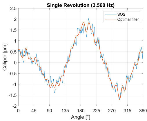
Figure 5: Comparison between the signal extracted by the SOS tool and the one extracted by the optimal filter.
