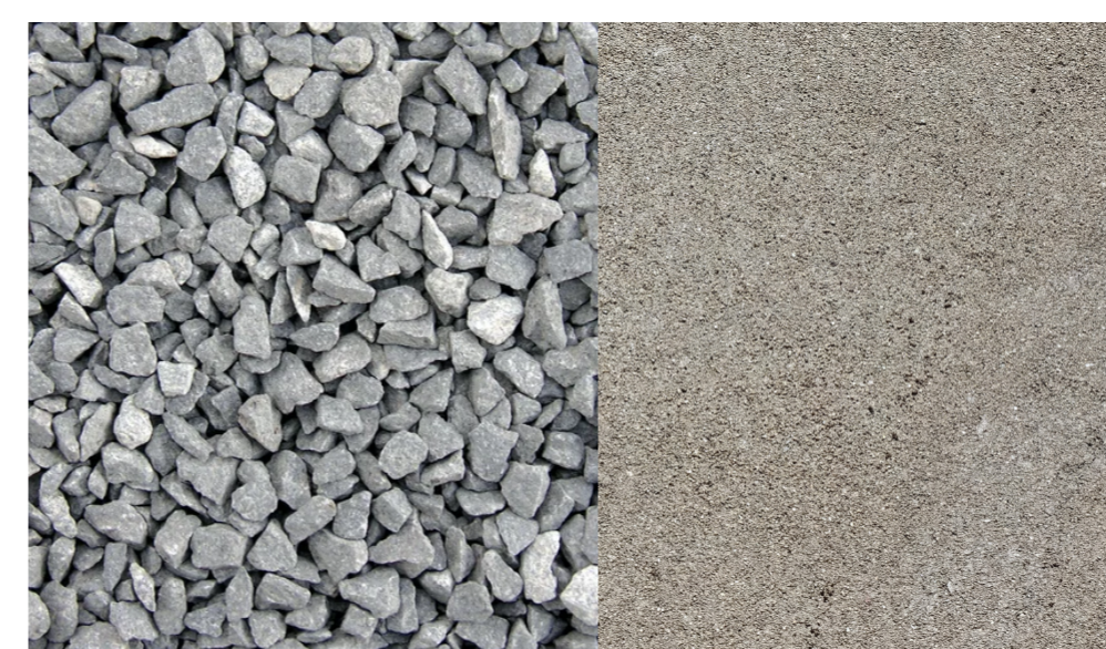
Screed made from recycled aggregates
