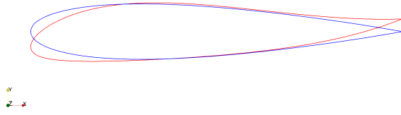
Figure 4: Comparison between NACA0015 (blu) and the optimized profile (red)
