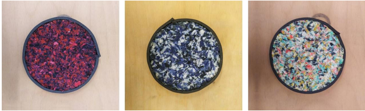
Figure 26. Absorption coefficient test samples, each consisting of 4-6 mm length fibers and each with the diameter \varnothing 10 cm (the sealing tapes cover test samples) (a) SC-4: Silk-based composite sample (b) CC-4: Cotton-based composite sample (c) VC-4: Viscose-based composite sample
