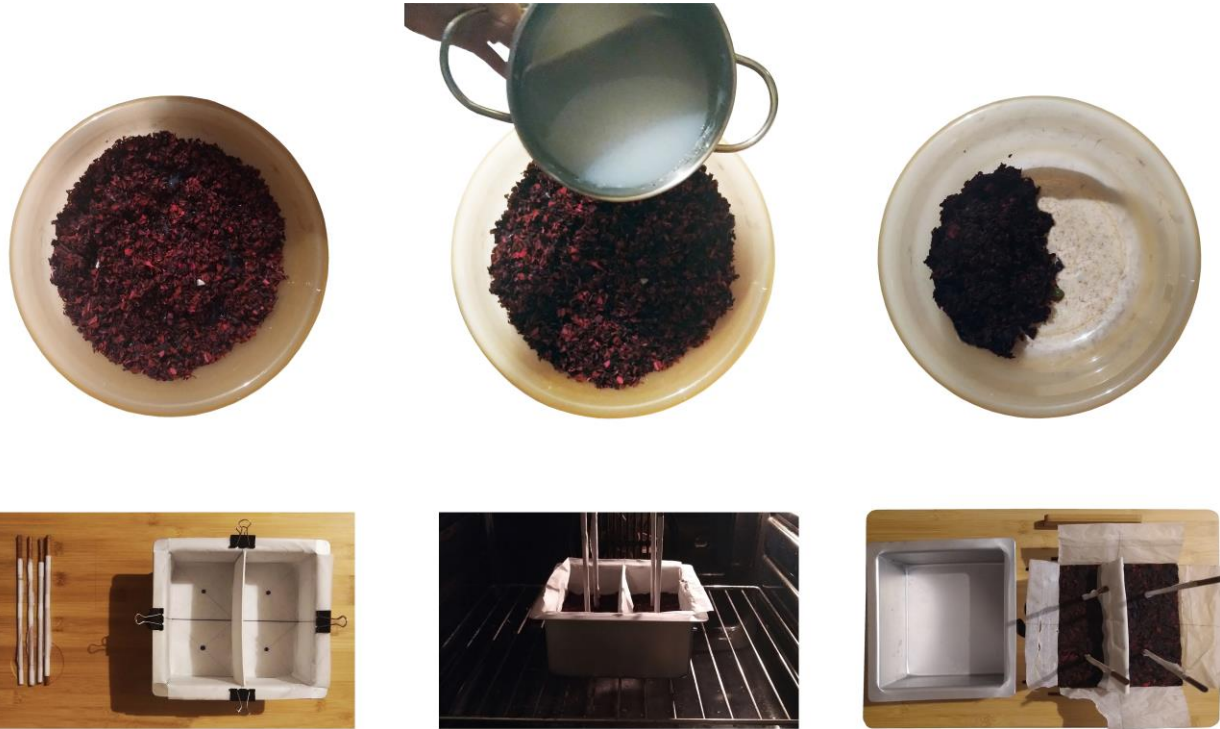
Figure 21. Production process of the silk-based bricks in Scale 1:2 (a) small-sized (4-6 mm) silk fibers (b) mixing the fibers with the starch-based binder (c) wet fiber-binder mixture (d) Square mold and the timber sticks for the holes (e) drying the silk-based bricks (f) removing them from the molds
