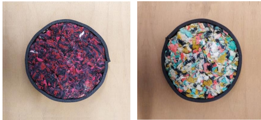
Figure 27. Sound absorption coefficient test samples, each consisting of 15-20 mm length fibers and each with the diameter \varnothing 10 cm (test samples are covered by the sealing tapes) (a) SC-5: Silk-based composite sample (b) VC-5: Viscose-based composite sample
