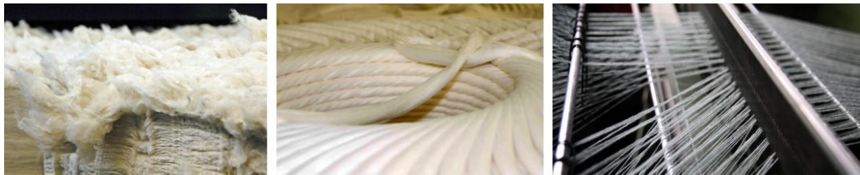
Figure 13. The production process of the cotton (a) Cotton fiber (b) Cotton yarn (c) Cotton weaving (Source: https://www.quilting-in-america.com/process-of-making-cotton.html ).
