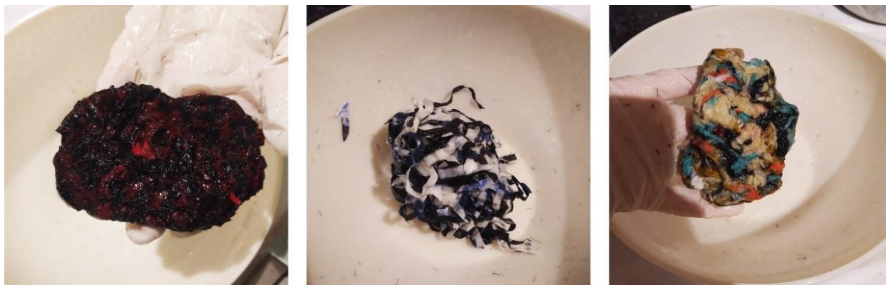
Figure 18. Fibrous blend (a) silk and starch-based glue mixture (b) cotton and starch-based glue mixture (c) viscose and starch-based glue mixture
