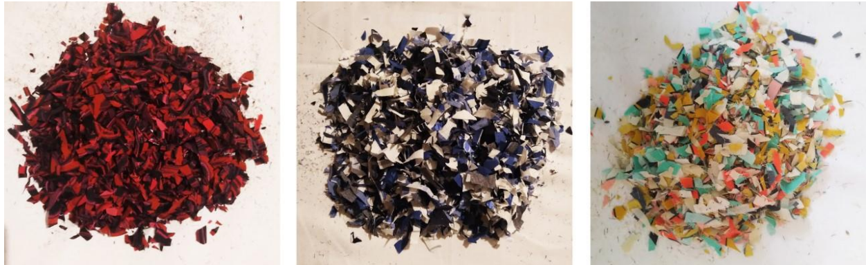
Figure 16. Fabric scraps fibers (a) silk waste (b) cotton waste (c) viscose waste
