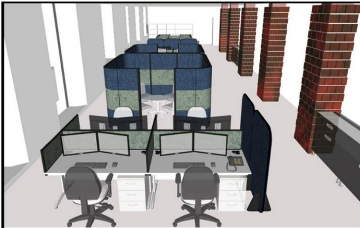
Meeting hubs made of panels (thickness: 80 mm) Brick form wall column cladding (thickness: 30 mm) Office desk dividers (thickness: 30 mm)
