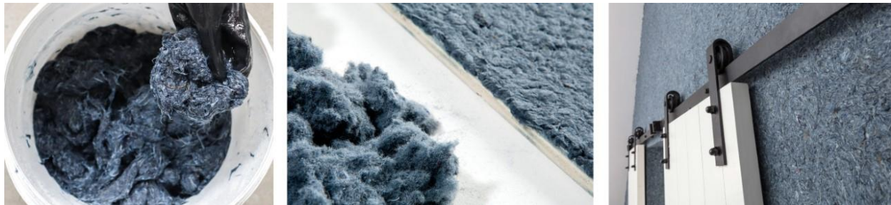
Figure 11. Wall panel made of recycled jeans fibers (Source: https://www.denimx.nl ).
