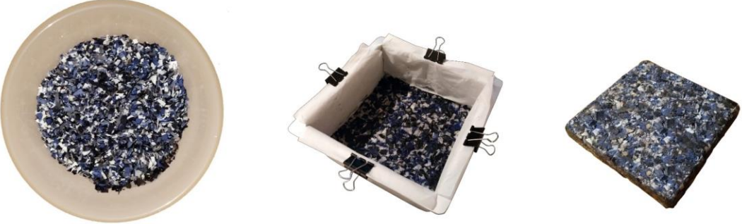
Figure 23. From fibers to the composite (a) small-sized (4-6 mm) cotton fibers (b) wet binder-fiber mixture in the square mold (c) cotton-based wall covering (150*150 mm)
