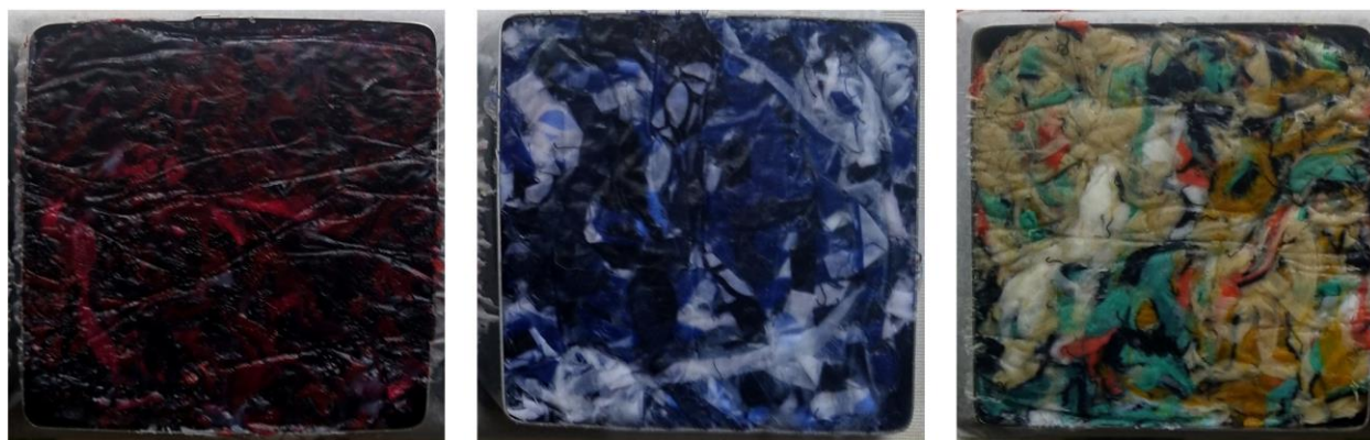
Figure 19. Fibrous blend in the square (80x80 mm) mold (a) silk-based blend (b) cotton-based blend (c) viscose-based blend.
