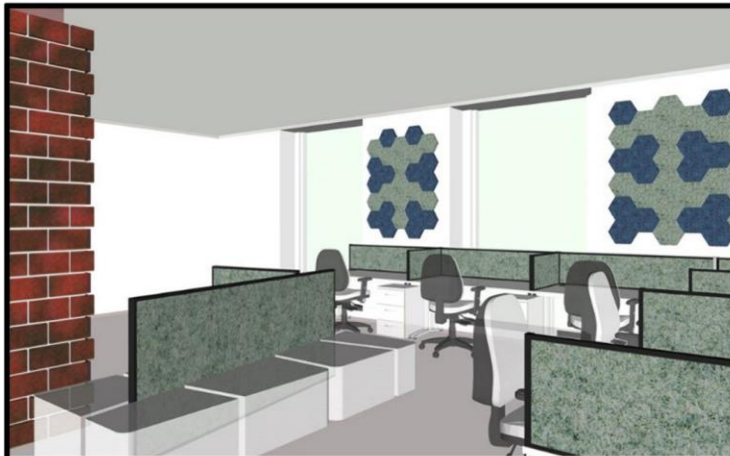
Hexagon shaped wallcoverings (thickness: 30 mm) Office desk dividers (thickness: 30 mm) Furniture dividers for silent working (thickness: 50 mm)
