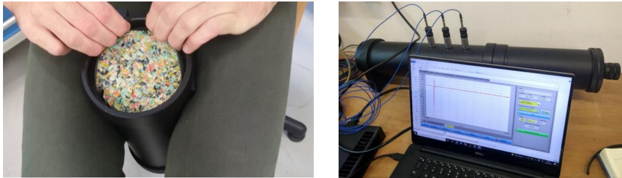
Figure 24. Sound absorption test area (a) The impedance tube and the software (b) Viscose-based composite sample (the diameter = \varnothing 10 ) is placed in the impedance tube
