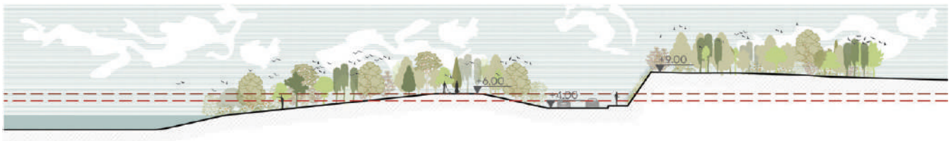
28. Cross section with lines of flooding risk
