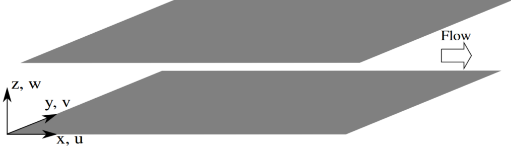
Figure 2.2: Definition of channel flow with reference adopted in the numerical code
