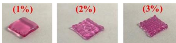
X. Alginate printed cubes fabricated with extrusion bioprinting. The concentration of alginate increases from left to right. 3% alginate concentration allows to obtain a more precise and porous structure [1].
