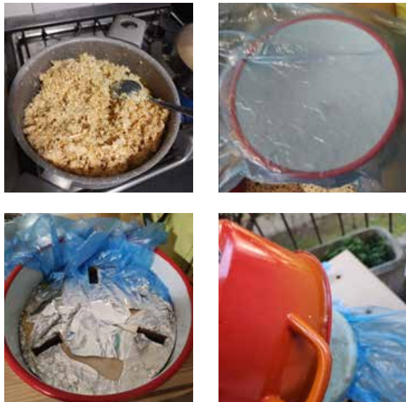
Image 90. Pressing and extraction of Stool's version 2 seat
