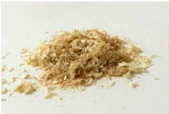
Image 60. Fibrous – sawmill, turning, brushing.
