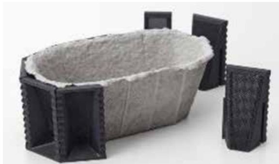
Image 38. 3D Printing moulds for recycled paper pulp products (Hayakawa, 2015)
