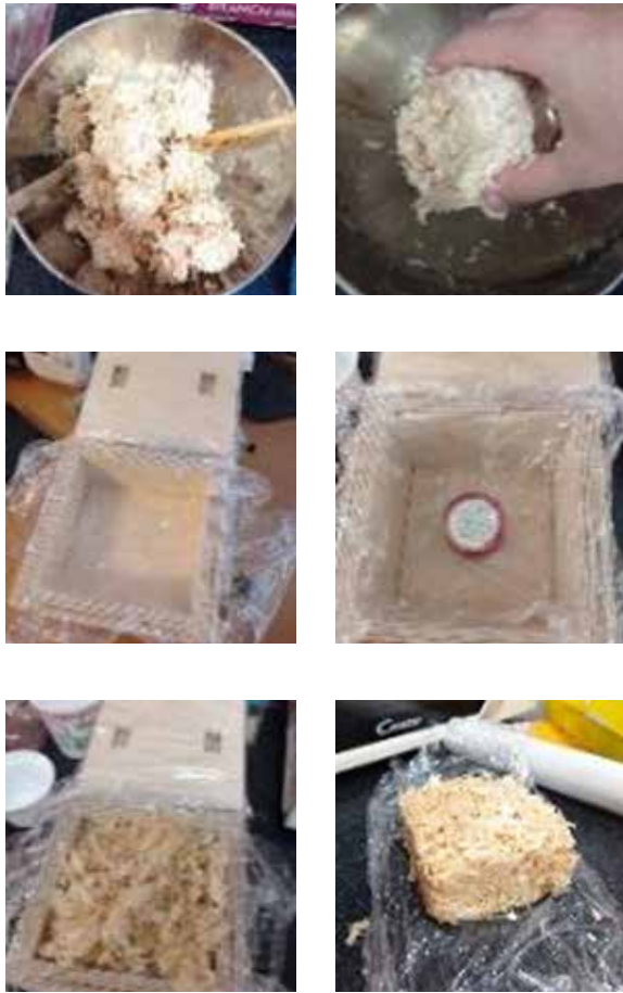
Figure 42. Process of recipe making and compression material with an inside shape - Packaging test
