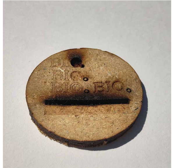
Image 68. Lasered sample 1 - Burned on the cut test
