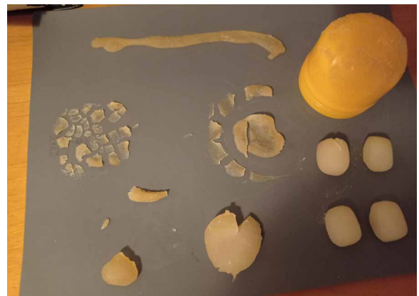
Figure 5. (1) Day one of the unmoulded recipe, moulded inside a cocoon like shape (2) Day three of unmoulded recipe inside a cocoon like shape, (3) More sugar base bioplastic samples day one, (4) More sugar base bioplastic day three
