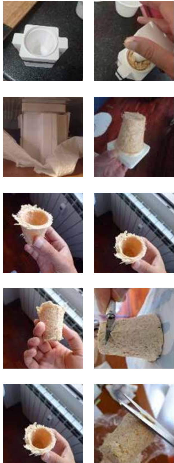
Figure 31. Replicating successful moulding process with corn starch + sawdust recipe for 3D printed moulded glass.
