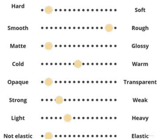
Figure 48. Property characterization for biomaterial proposed
