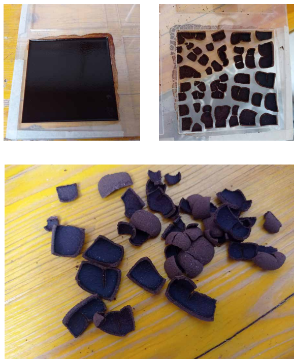
Figure 7. Samples of agar-agar coffee base bioplastic
