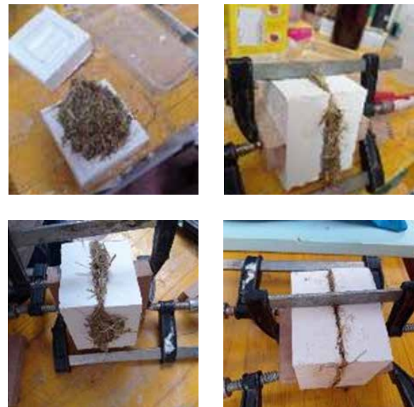
Figure 25. Moulding grass + corn-starch recipe, process experimentation
