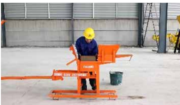
Figure 33. (China Brick Machines, 2021) Brick machine production process. 1) Pouring brick powder 2) Placing brick powder on the compression compartment, 3) Pull lever to compress, 4) Pull out brick.
