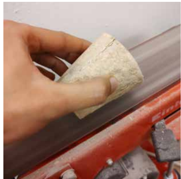
Image 65. Insulator cup sanding process
