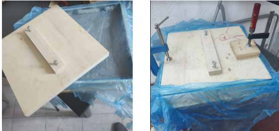
Image 55. Complete sheet compressing mold, Pressed sheet compression mold.
