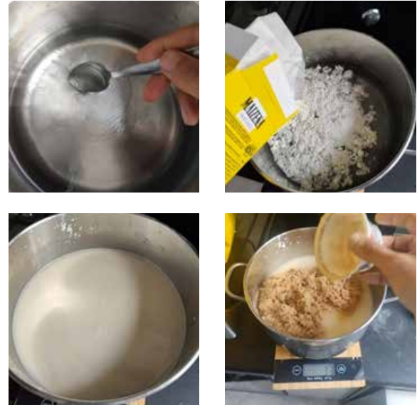
Image 85. Seat stool biomaterial preparation where everything is mixed and then heated.
