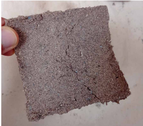
Figure 14. Corn starch + sawdust sample after drying process (APPENDIX B – Recipe 5.1)
