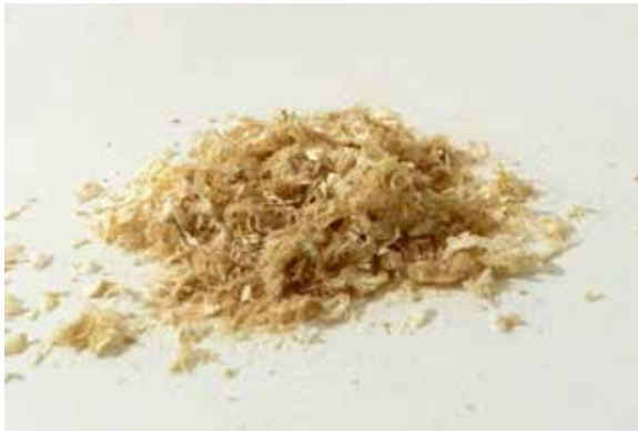
Image 59. Mid-size – brushing, cutting, turning (mixed fine + fibrous).
