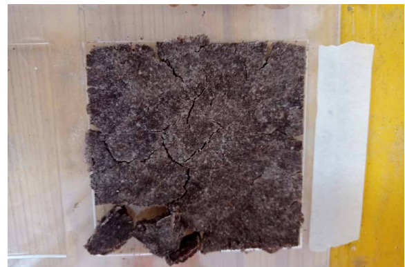
Figure 8. Agar agar + MC Coffe recipe after drying process.
