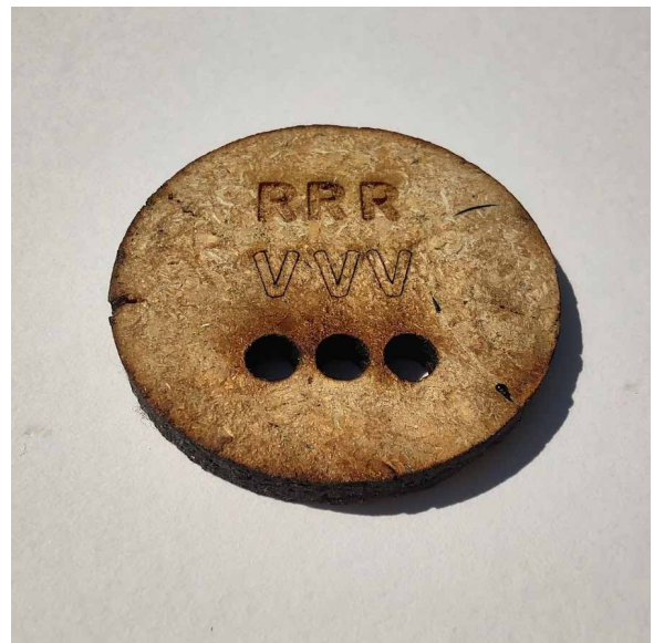
Image 69. Lasered sample 2, clean cut, raster and vector engraving
