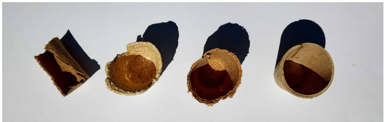
Image 102. (1) Isolator cup with particle sawdust compression moulded. (2) Evolution of cups samples and tests until the end result
