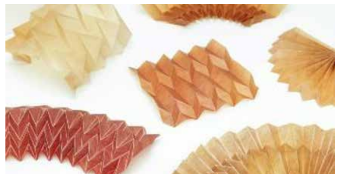
Image 19. Examples of biomaterial products made through folding: (1) Karagenina base bioplastic folded prototype (Pacheco & Márquez, 2020) (2-3) Lionne Van-Deursen's UNFOLD project samples composed of bacterial cellulose and finished through folding (Van-Deursen, 2020)
