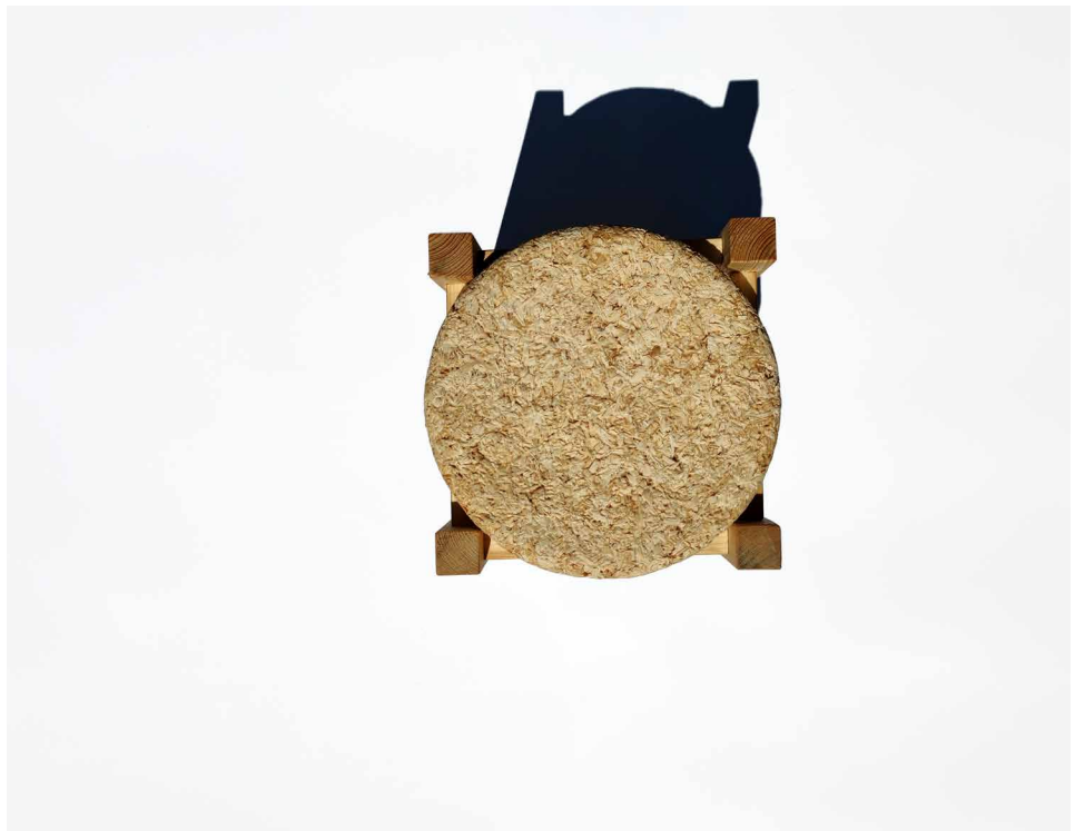
Image 107. (1) (3) Biomaterial seats (1 of fibre sawdust, 2 mixed powder and fibre sawdust) Version 2 Biomate- rial Stool
