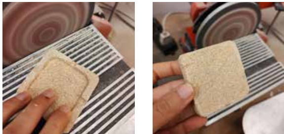
Image 61. Pressing, drying and sanding of the ashtray piece prototype.
