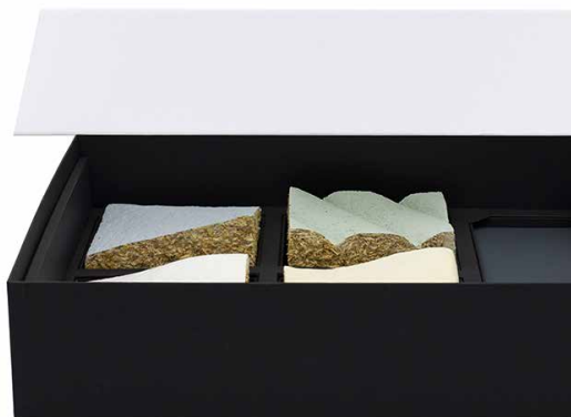
Image 10. Section views of the isolating panels samples made of mycelium (MOGU, 2022)
