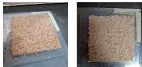
Figure 15. Sodium alginate + sawdust recipe after drying process (APPENDIX B – Recipe 4.5)
