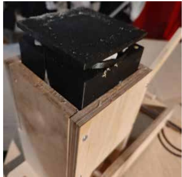
Image 50. Mold not fitting in the machine.
