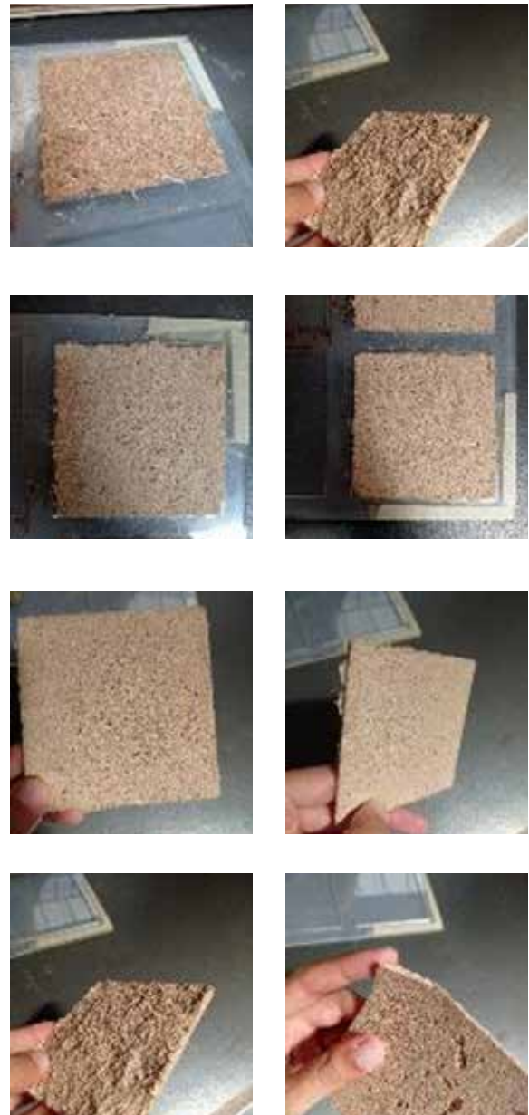
Figure 16. Views of CMC + sawdust samples after drying process (APPENDIX B - Recipe 10.1)
