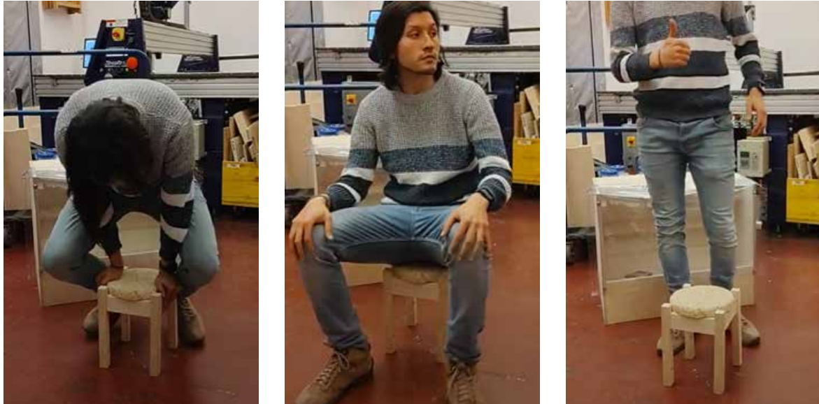
Image 95. Function and resistance test of finished stool
