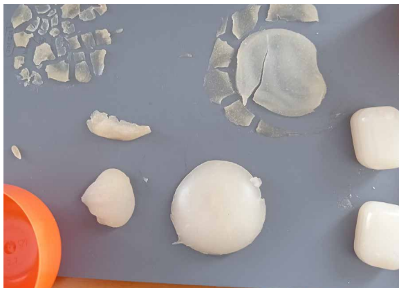
Figure 5. (1) Day one of the unmoulded recipe, moulded inside a cocoon like shape (2) Day three of unmoulded recipe inside a cocoon like shape, (3) More sugar base bioplastic samples day one, (4) More sugar base bioplastic day three
