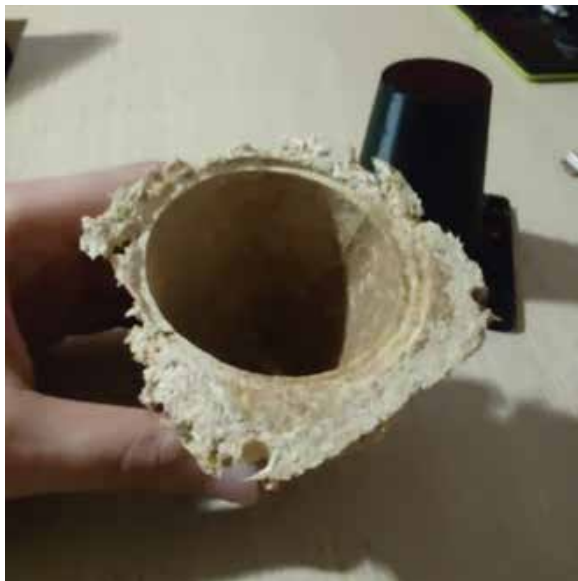
Image 64. Thermal insulator cup drying and mold extraction.
