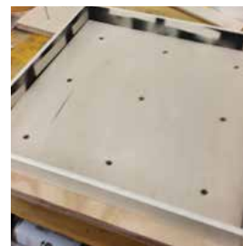
Image 54. Milling of base 1, Milling of containing frame, Assembled base, Holes for piston assembled
