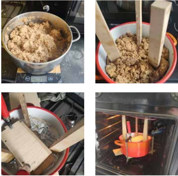
Image 86. Embedding of legs and cooking of biomaterial seat stool
