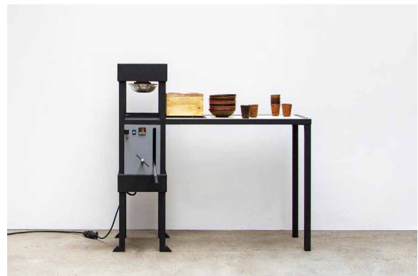
Image 16. Heat compression moulding machine by Precious Plastics and their project Beyond Plastics (Precious Plastics, 2020)
