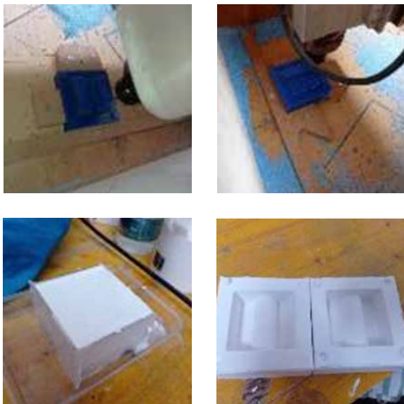
Figure 24. Clay moulding manufacturing process
