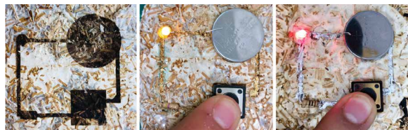
Image 21. Laser cut and engraved mycelium block used as replacement for a protoboard case (Lasaro Vasquez & Vega, 2019)
