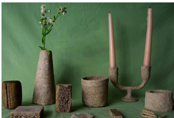
Image 22. Examples of milled biomaterial blocks made of nutshells, from the design studio Keep Life (Keep Life, 2022).
