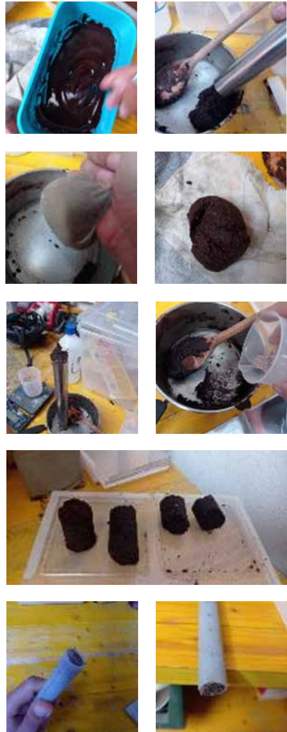
Figure 21. Extrusion experiments with sodium alginate + coffee recipe (1) Initial mix, (2) Extrusion process, (3-4) Sieving process, (5-7) Extrusion process 2, (8-9) Extrusion process with sawdust.
