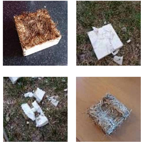
Figure 26. Drying and unmoulding procedure for grass + corn-starch
