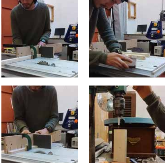
Image 92. Cutting legs to measure, sanding pieces and opening dowel holes.
