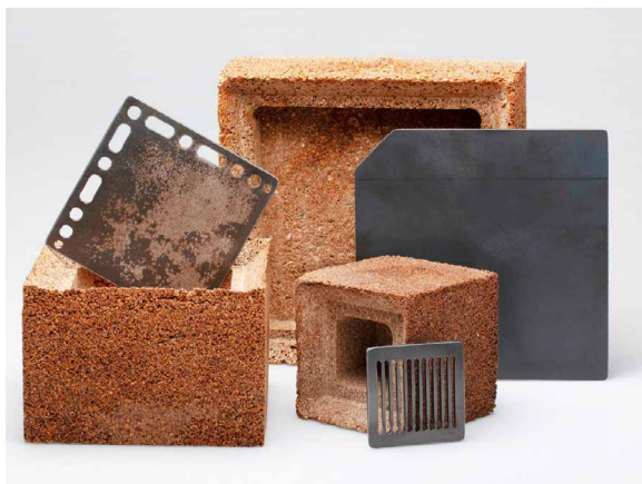
Image 22. Examples of milled biomaterial blocks made of nutshells, from the design studio Keep Life (Keep Life, 2022).
