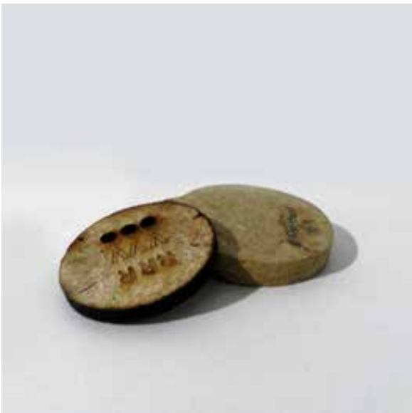
Image 67. Lasering tests with the sawdust biomaterial
