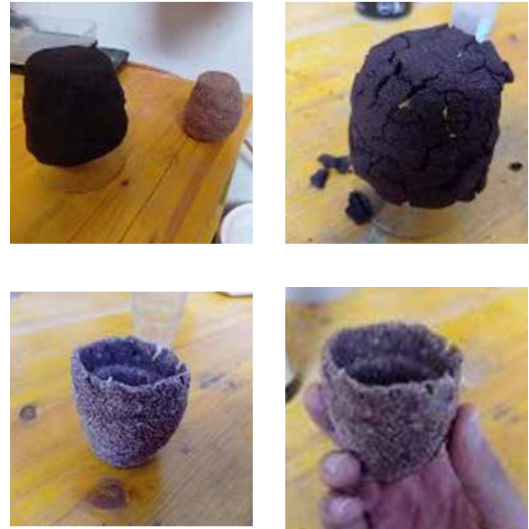
Figure 20. (1-2) Moulding glass process with corn starch + coffee recipe, (3-4) Moulding small glass process with corn starch + sawdust recipe.
