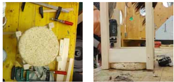
Image 93. Clamping, joining and pre-drilling to assemble whole stool.
