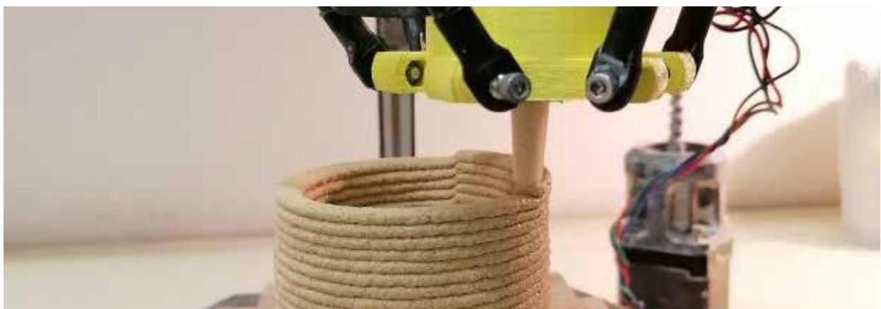
Image 18. Example of 3D printing solutions suited for biomaterials: (1) 3D Hydraulic machine suited for viscous liquids (3D Potter, 2022), (2) Tinkered biomaterial 3D printer (EDDM, 2020), (3) Ana Otero 3D printing biomaterial prototype based out of egg shells, (Otero, 2022)
