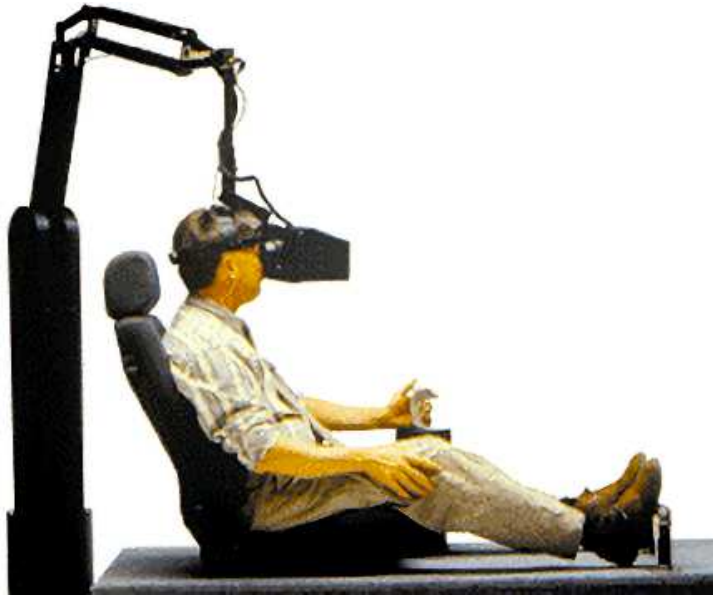
Figure 1-32 A mechanical tracking device developed by Fake Space
