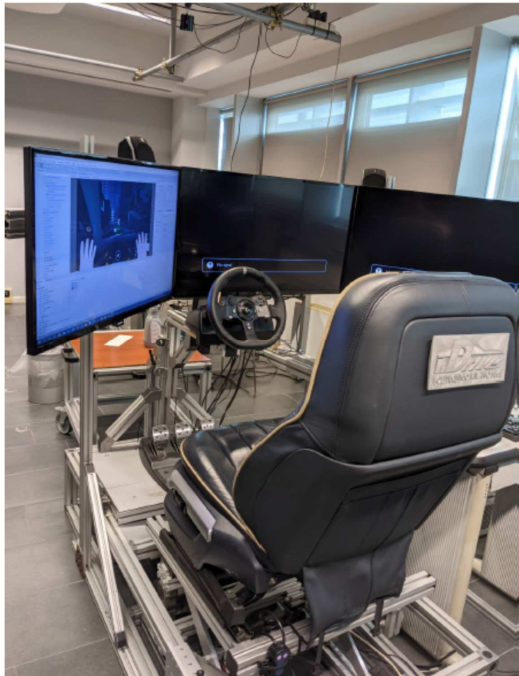
Figure 5-1 iDrive simulator (source Dadhich et al. [178])
