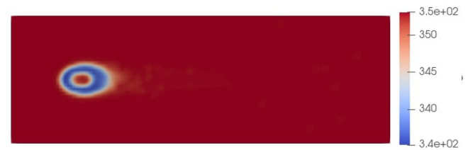
Figure 5: Wall temperature distribution Bai 80 °C
