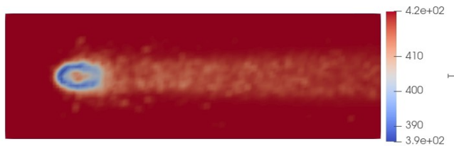
Figure 8: Wall temperature distribution Kuhnke 150 °C
