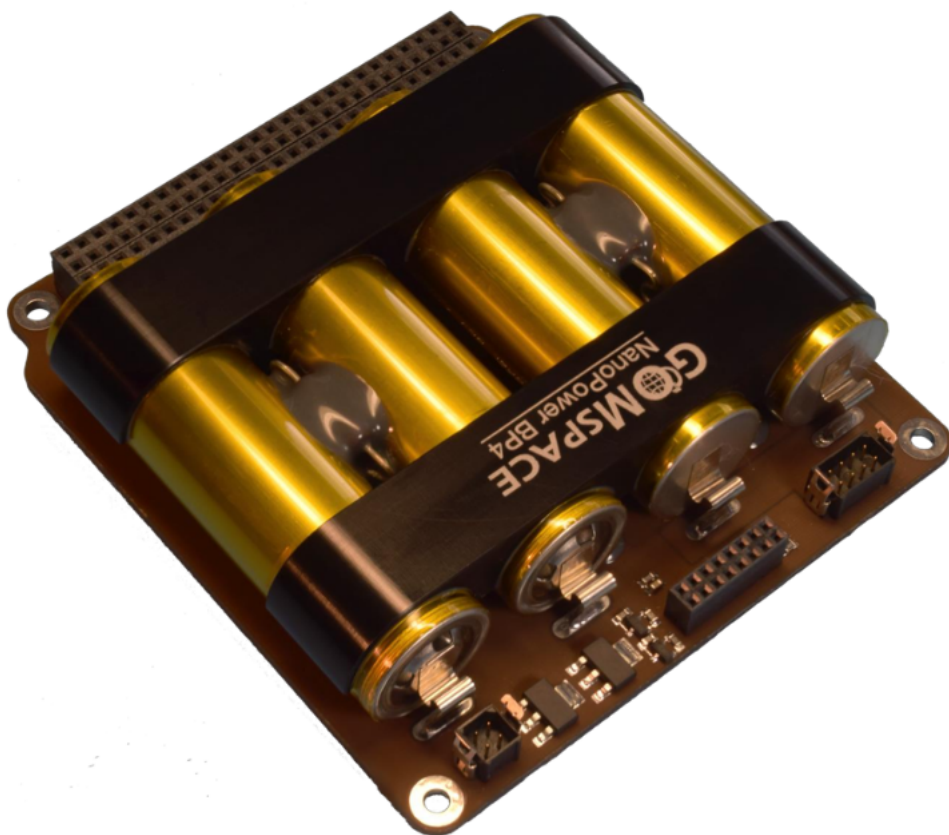
Figure 2.1: NanoPower BP4 from GomSpace.
