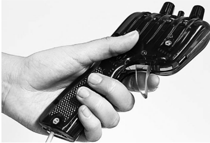
Figure 1.4: An example of handset control for real time discomfort acquisition used in the research [17] [18]
