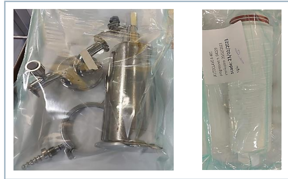
Figure 27 - Reservoir : housing and filter
