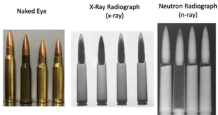
Figure 1.19: Neutron and X-ray radiography of four bullets. One of them has a different internal structure which cannot be distinguished in the second image as X-ray are equally attenuated. The neutron radiography yields different, yet complementary, information to x-ray radiography.
