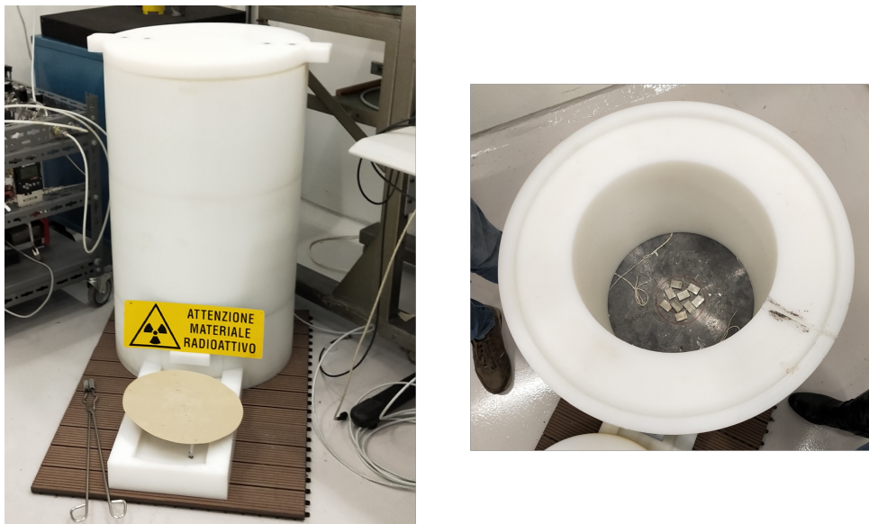
Figure 2.3: Thermalized neutron source held at Politecnico di Milano. On the left it is possible to observe the external polyethylene cylinder used to thermalize neutrons emitted by the Am-Be source contained inside, as well as to shield radiations. While, on the left, the lead disk is visible together with some neutron detectors.
