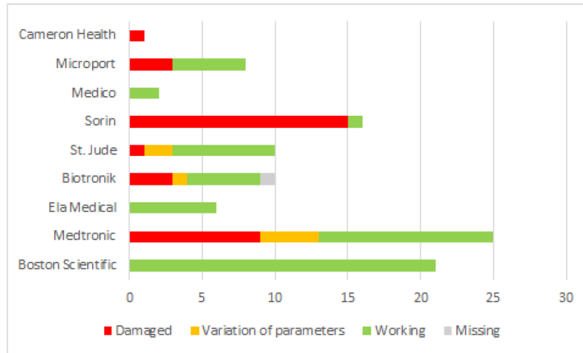
Figure 1.17: Bar chart summarizing the information obtained after the neutron radiography performed on 99 CIEDs at the NEUTRA facility. The diagnosis system reported that almost 30% of the interrogated devices were damaged, while in less than 10% there was a variation of working parameters or a sensible decrease in battery life [53].
