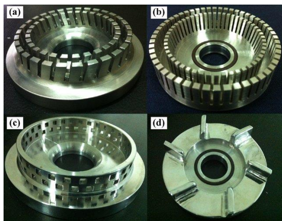
Figure 1.11 Geometric details of (a and c) the stator and (b and d) the rotor in (a and b) the teathed and (c and d) the blade-screen in-line high-shear mixers [46] .
