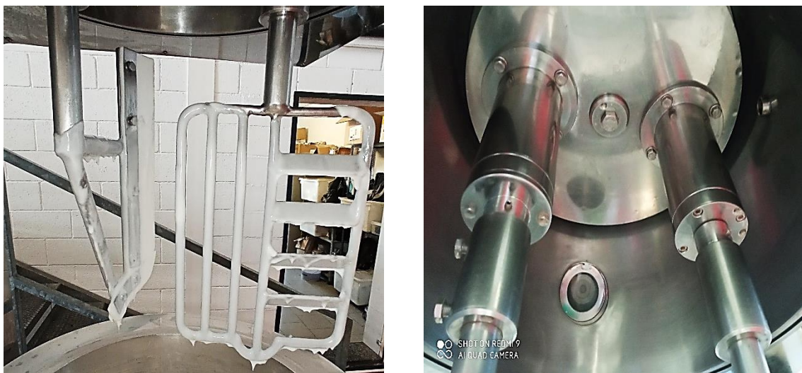
Figure 5.5 Details of the mixing system: structure of the counter-rotating blade and scraper (left) and their detached crankshafts (right); personal processing (directly taken on the field by the author).
