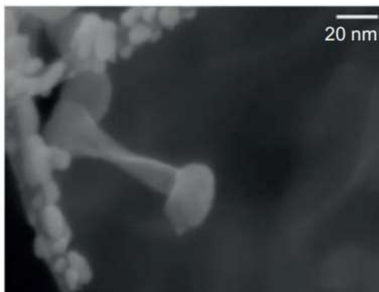
Figure 1.28 - SEM image showing carbon filament with catalyst particle at its end.
