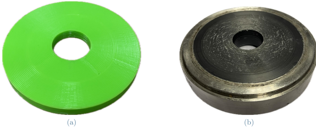
Figure 4: Fuel grains: (a) ABS and (b) Paraffin-based.
