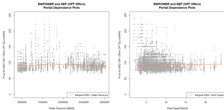
FIGURE 7.12: Cluster of Thermoelectric PUs from ENIPOWER and S.E.F., MSD OFF bids: visualization of marginal effects via Partial Dependence Plots of the variables Water Reservoir (left) and Wind Speed (right).
