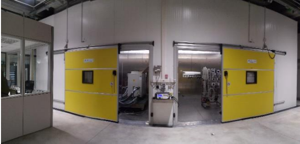
Figure 1: RELAB 50(kW) climatic chambers to simulate external and internal environments.
