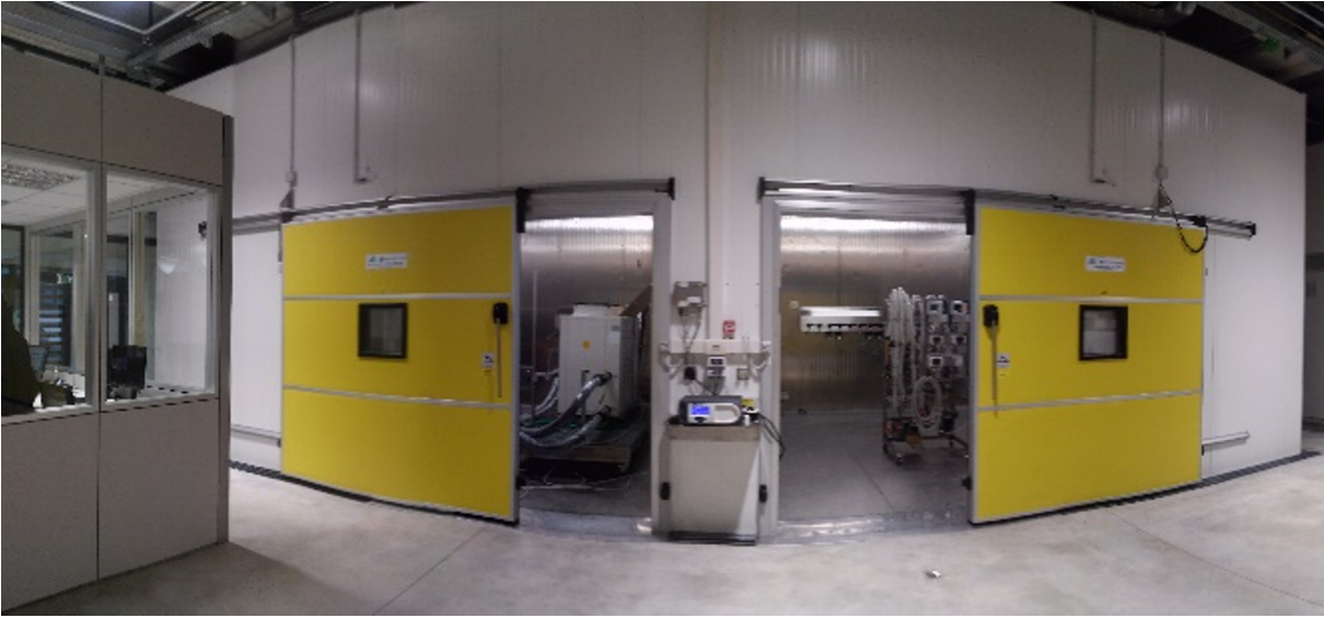
Figure 4.3: ReLab 50 (kW) calorimeters to simulate external and internal environments
