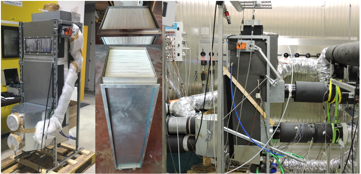
Figure 4.4: 1) on the left the test rig that contains the heat exchanger the humidifier and the air to water heat exchanger, 2) in the center the tested air to air heat exchanger, 3) on the right the test rig attached to the measuring tubes and the two fans
