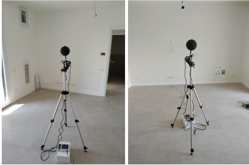
Figure 3.6: Indoor globo thermometer positioned in the center of the living room. The two pictures are the two sides of the empty living room. The instrument accuracy is \pm 0.23 ( ^{\circ}\text{C} )
