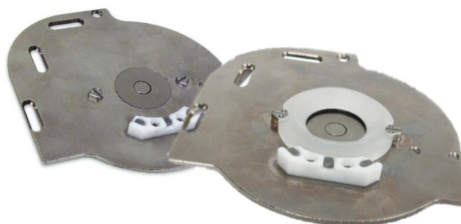
Figure 4.4: Keysight's sample plates. The sample plate in the left part is used in the air: the sample can be fixed by the two clamps to get stability and ease of use. The sample plate in the right part of the picture serves the purpose for the electrochemical measurements: the sample is mounted in the Teflon EC-cell and a Viton O-ring is used to seal and to avoid any leakage of liquid. The WE, RE and CE are inserted in the three outlets in the white holder. By using magnetic suspension, loading becomes more convenient and mechanical drift is eliminated [120].
