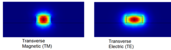
Figure 2.6: In TE mode the evanescent field is less confined at the top and bottom of the core; however, in TM it is the opposite.
