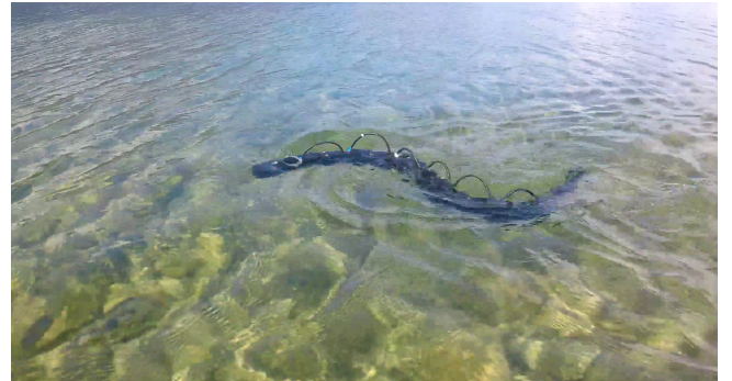
Figure 15: The robot performing lateral undulation during experimental tests
