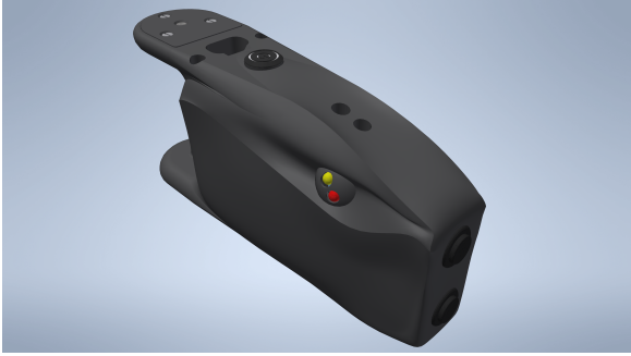
Figure 5: The head of the aquatic snake robot
