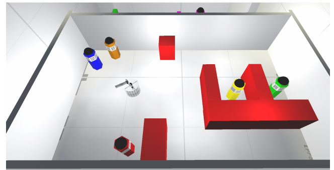
Figure 5: Simulation of our system. The white cylinder with an arm is Virtual Odile, the prisms are Stations.
