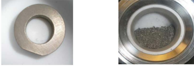
Figure 35 - Magnetic components before and after exposure to hydrogen
