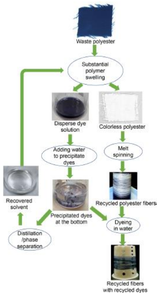
Figure 16: Recycling of PET and disperse dyes from waste textiles, Mu et al. (2023)
