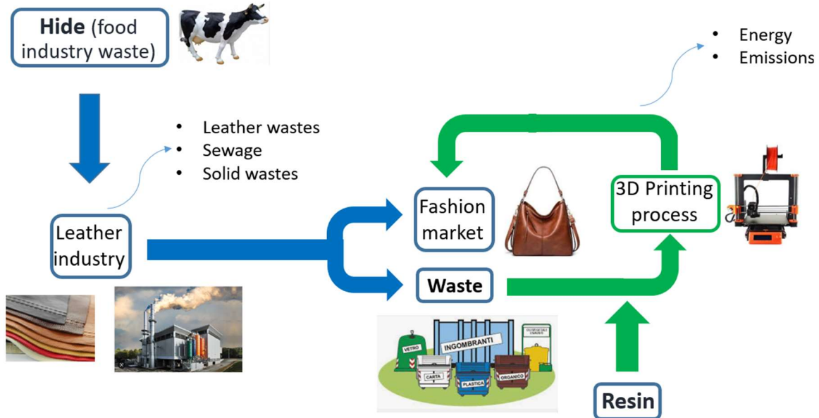
Figure 30: Graphical scheme of linear industrial leather production (blue) and circular 3D Printing with leather waste production (green).
