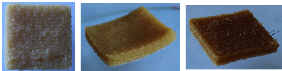
Figure 80: Results of 3D printed sample after: printing (left), curing (middle); drying (right).
