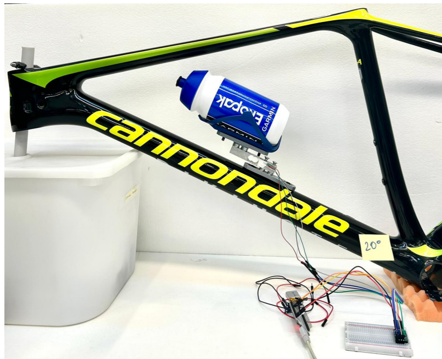
Figure9: Test Bench with MTB frame, first measurement in a semi-real condition
