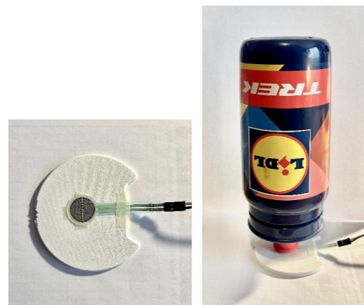
Figures 6 and 7: First Trial 1.1 for validate the sensor - Using FRS 20 mm diameter
