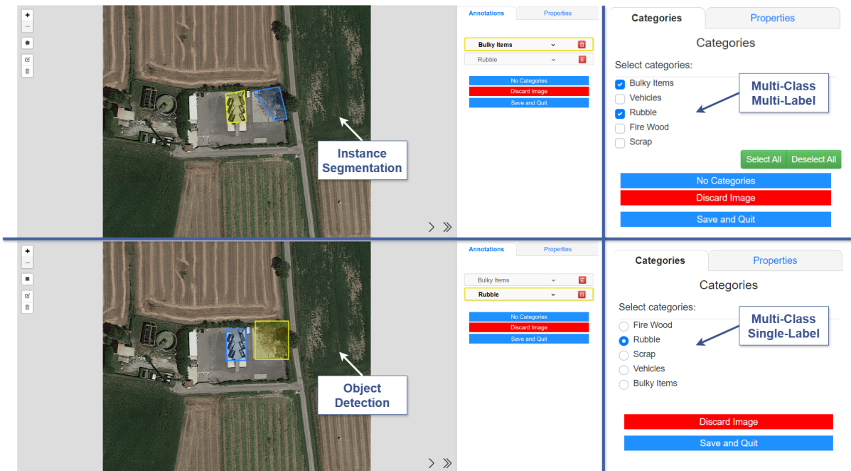
Figure 5.13: Annotator: annotation interface for instance segmentation, object detection, multi-class multi-label classification, and multi-class single-label classification.
