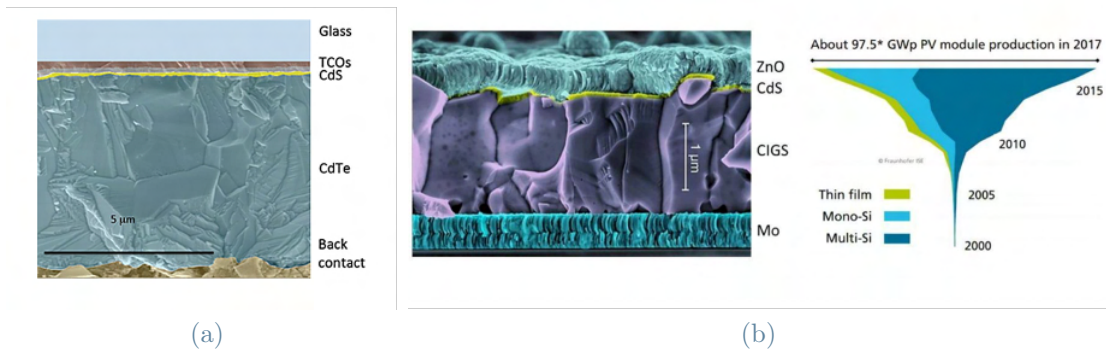
Figure 2: Examples of PV application of thin films (a) and world production of different types of PV (b). Fig.taken from [2]
