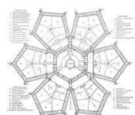
Plan of Millbank Prison: six pentagons with a tower at the centre are arranged around a chapel.
