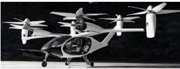
Figure 2. Joby Aviation S4: example of tilt wing/rotor eVTOL model. Source: jobyaviation.com
