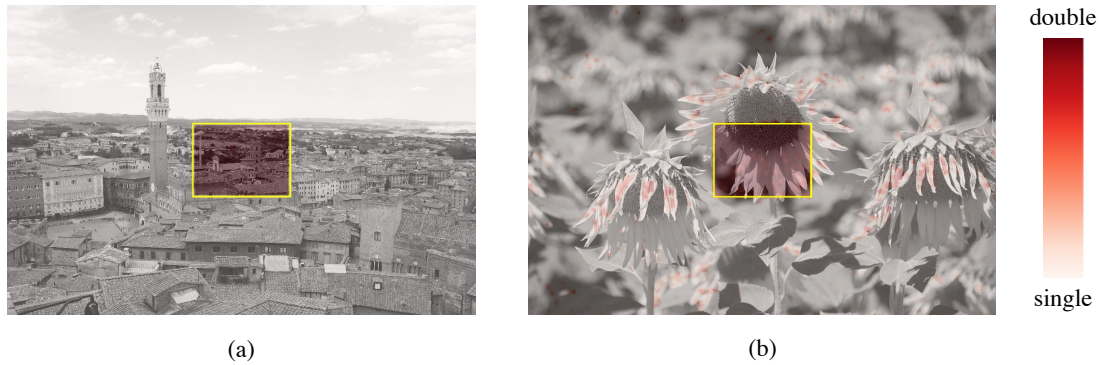
Figure 3.10: A-DJPEG (a) and NA-DJPEG (b) localization example of a compressed central region with QF2 = 95 and QF1 = 80 . C_{hist} is used for the aligned case while C_{noise} for the non-aligned case. Actual forged region lies inside the yellow rectangle.
