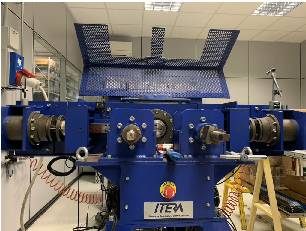
Figure 3.3: Experimental Set Up Roller Bearing - 1
