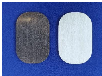
Figure 4.13 - CFRE (left) and GFRE (right) samples before palladium coating
