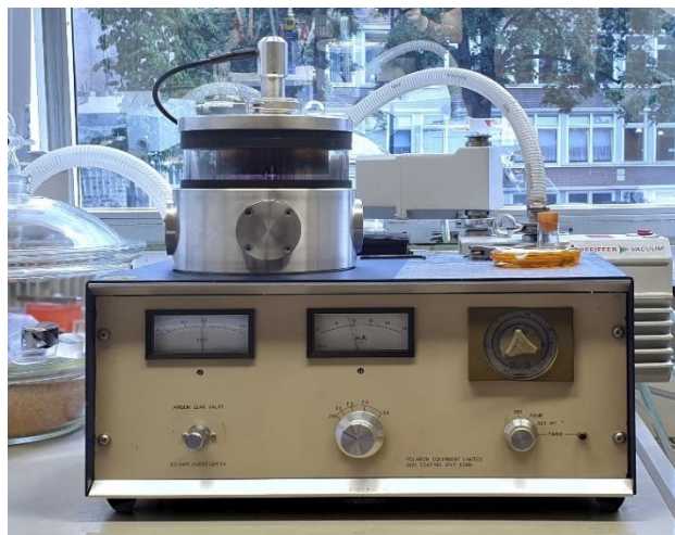
Figure 4.14 - Sputtering machine used for palladium coating deposition
