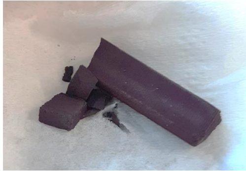
Figure 74 - Brown specimen after debinding treatment.
