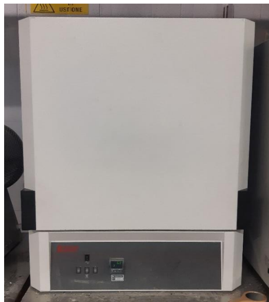
Figure 59 - Lenton furnace in which thermal treatments were performed.
