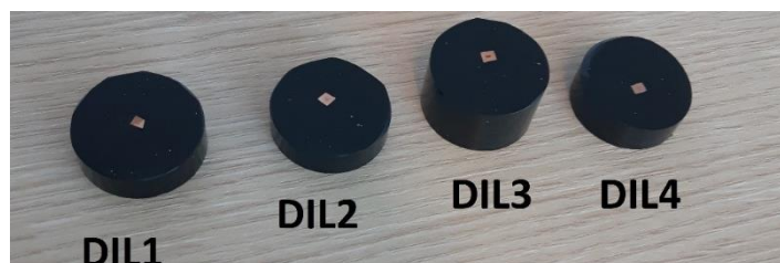
Figure 55 - Resin embedded brown specimen for SEM analysis.
