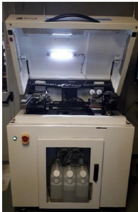
Figure 44 - ExOne Innovent+ binder jetting printer.
