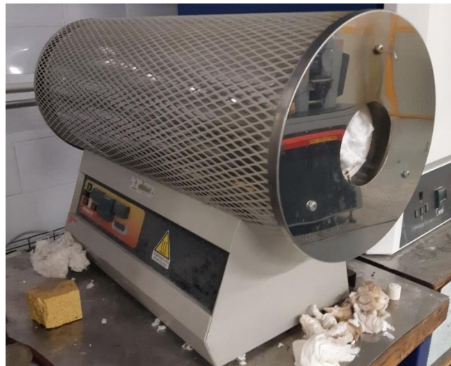
Figure 49 - Carbolite tube furnace.
