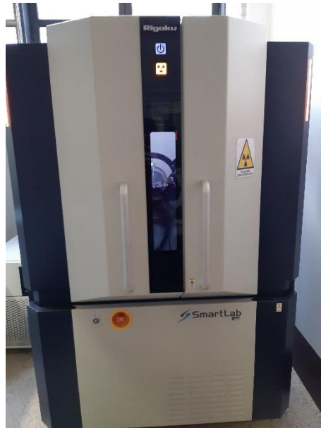
Figure 43 - Rigaku SmartLab X-ray diffractometer.
