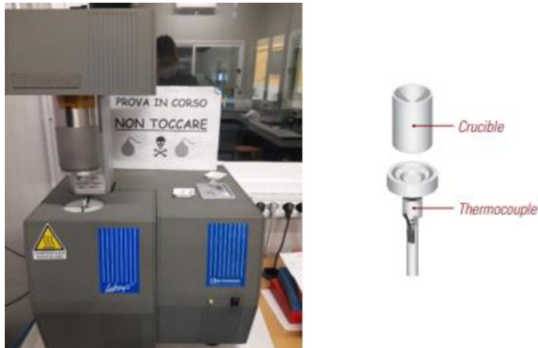
Figure 50 - Setaram Labsys device (left) and alumina crucible used to perform the test (right).
