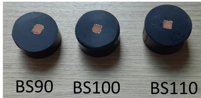
Figure 58 - Resin embedded sintered specimens.
