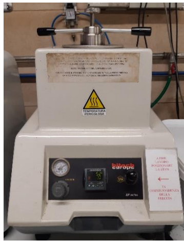
Figure 38 - Hitech Europe EP15 pneumatic mounting press.
