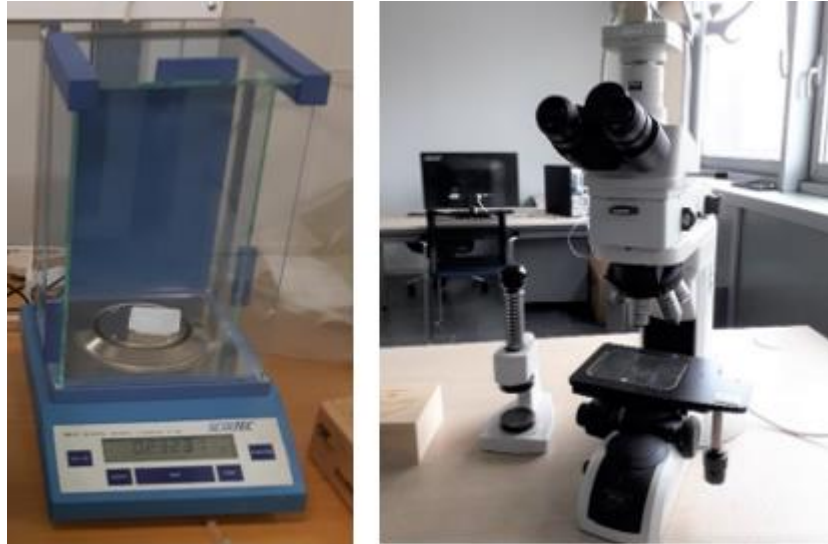
Figure 48 - Scaltec SBC 22 electronic scale (left) and Nikon Eclipse LV250NL optical microscope (right).
