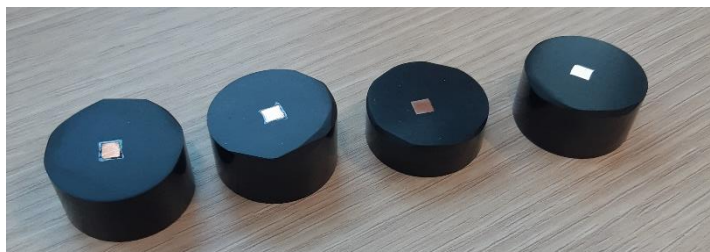
Figure 62 - Resin embedded sintered specimens for SEM analysis.
