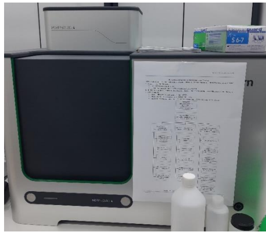
Figure 34 - Malvern Panalytical Morphologi 4 automated imaging analyzer.
