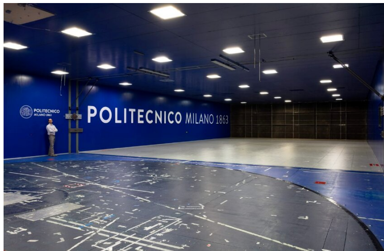
Figure 6.2: Boundary layer test section
