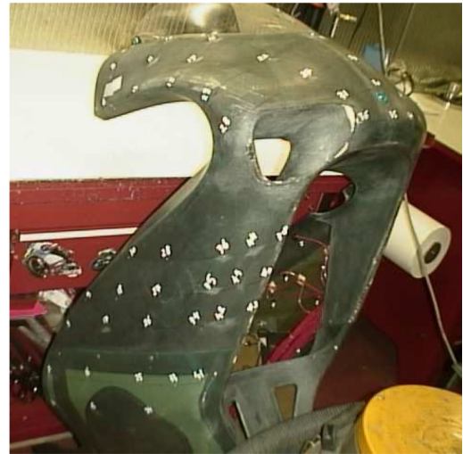
(b) Experimental setup for pressure field measurement on frontal fairings
