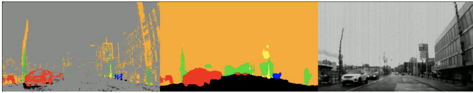
Figure 5.8: A sample taken from the DDD17 dataset. On the right side is the gray-scale image generated by using 50ms of APS data. In the middle is the corresponding labels image generated using a pre-trained CNN. By integrating over the same time interval, we can obtain an image reconstruction using the events provided by the DVS sensor. Each event is assigned the value of the corresponding pixel of the labels reference image.
