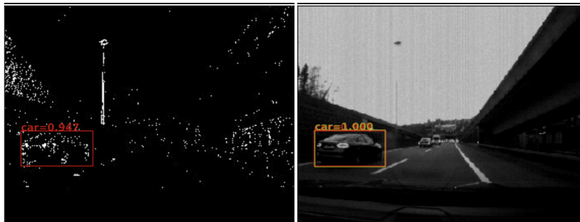
Figure 4.8: Output of the detection pipeline proposed by Chen [81]. The left image of is the DVS image with bounding boxes (in red) produced by DVS-only detection, while the right image of each pair is the APS image with DVS-only bounding boxes (in red) copied over and the RCC detections (in yellow) for comparison.
