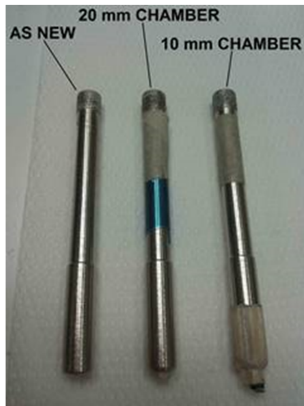
Figure 3.2: Modified micro corers [36] - Courtesy of Leonardo.
